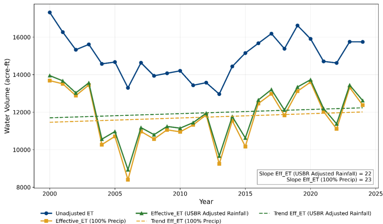
Figure A2: Annual Unadjusted and Effective ET for Levee Zones within ABCWUA, 2000-2024.
