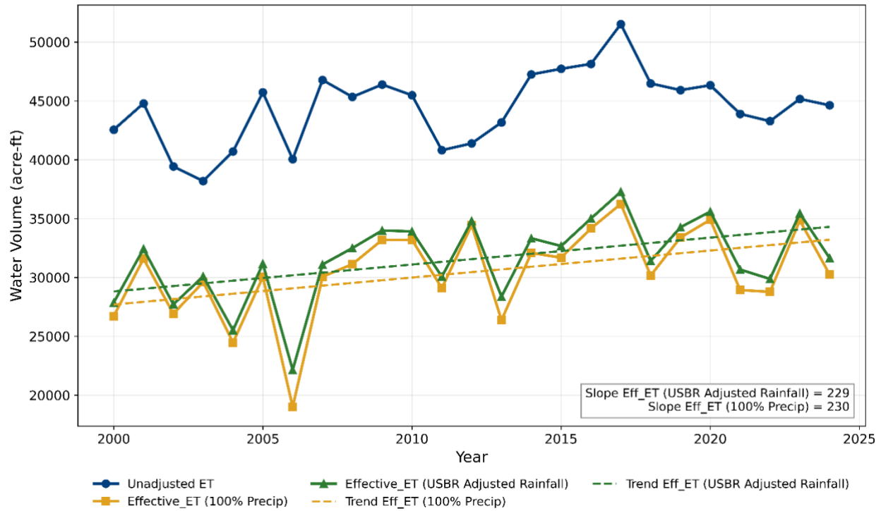
Figure A8: Annual Unadjusted and Effective ET for MRGCD-Intersected Areas in the BDANWR, 2000-2024
